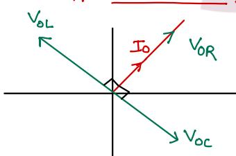
Phase difference b/w  $V_{OR}$  &  $I_0$  zero.
