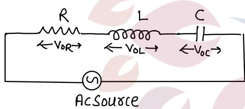
Suppose there are resistance (R), inductance (L) & capacitance (C) connected in series with applied AC source.
