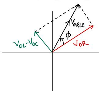
→  $V_{ORLC}$  leads current by  $\phi$  angle.
