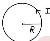
Let we have a current carrying coil of radius ( $R$ ). self-inductance of coil is  $L$  and no. of turns in coil is  $N$ .
