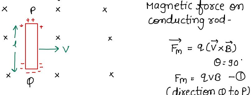
→ This force acts on free  $e^-$  of rod. Electron being negative charge feels force in P to  $\phi$  direction. Due to which
