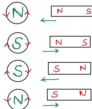
Lenz's Law states that induced current always opposes the cause. This means that when electric energy is produced, some other force must be doing work that is converted into electrical energy.
