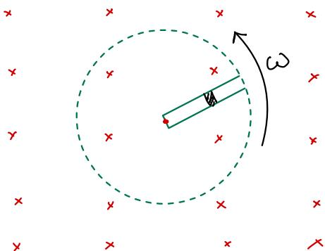
Let we have rod of length 'l'. angular velocity ( $\omega$ ) and rod is rotating in Uniform magnetic field ( $B$ ).
