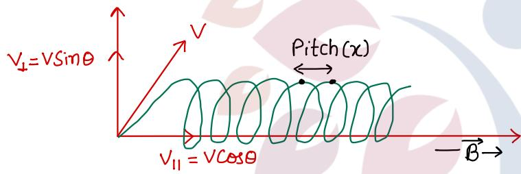
Suppose we have a charged particle of charge  $q$ , moving with velocity  $v$  in magnetic field  $B$ . Angle b/w velocity & magnetic field is  $\theta$ .
