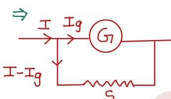
$$\begin{aligned} I_g G_i &= (I - I_g)S \\ I - I_g &= \frac{I_g G_i}{S} \\ I &= \frac{I_g G_i}{S} + I_g \\ I &= \frac{1 \times 10^{-3} \times 99}{1} + 1 \times 10^{-3} \\ I &= \end{aligned}$$
