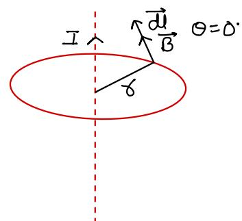
Suppose there is a current carrying conductor of  $\infty$  length. Current  $I$  is flowing through it. To calculate magnetic field we assume a circular amperian loop around wire of radius small  $x$ .
