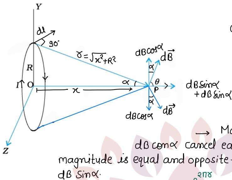
Let we have a current carrying circular loop of Radius R. At point P situated on axis of loop at distance x from center of loop. Angle b/w  $\vec{R}$  &  $dl$  is  $90^\circ$ . So,  $\sin\theta = \sin 90^\circ = 1$ .
