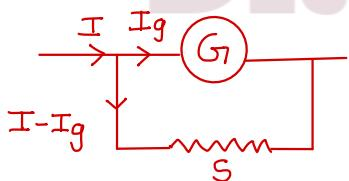
By joining a shunt resistance of very less value in parallel combination with Galvanometer.
