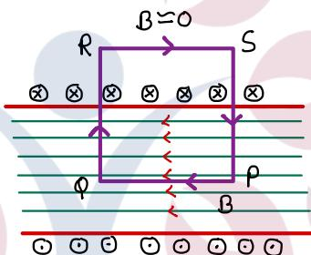
→ Let a solenoid of radius  $R$  & length  $L$ , whose length is very large than its radius. There are  $n$  turns per unit length and current  $I$  is flowing through it. Let  $B$  is magnetic field produced by it.
