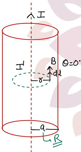
Let we have a current carrying wire of Radius ( $a$ ). Current ( $I$ ) is flowing it. To calculate Magnetic field. we assume amperian loop of radius ( $r$ ).
