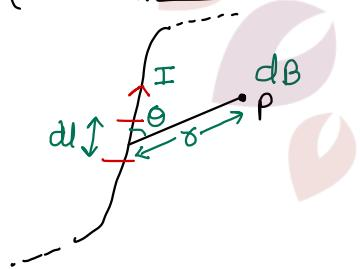
According to this law, produced magnetic field at a point P ( $\sigma, \theta$ ) due to current element ( $Idl$ ) -
