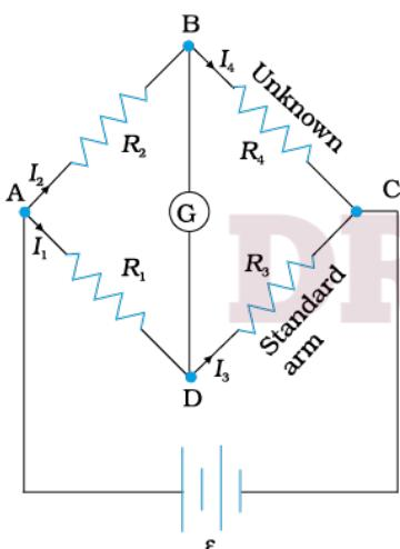
→ In balanced conditions resistor are such that there are no current through Galvanometer.
