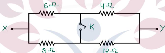
1. when Key is open:-  $R_1 = 6\Omega$  &  $R_2 = 4\Omega$  are in series
