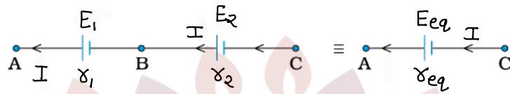
combination of cells in which one terminal of a cell is joined with opposite terminal of 2<sup>nd</sup> cell, is known as series combination.
