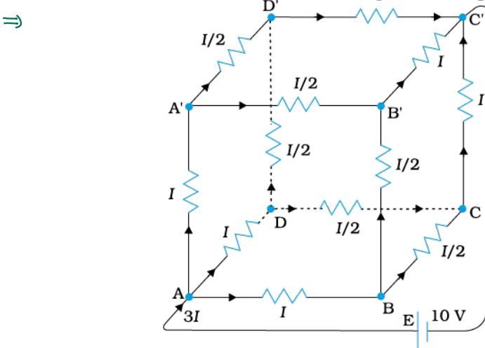
→ This network is not reducible to a simple series and parallel combination of resistors.
